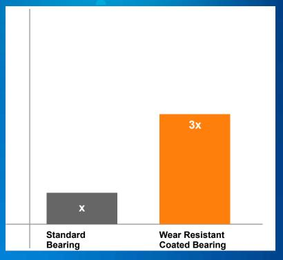
**Roller Bearing Endurance Test Comparison**
