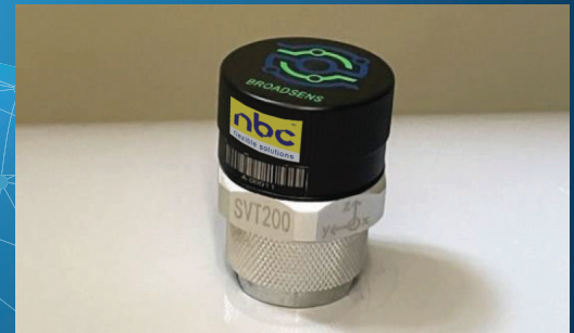
Wireless vibration & temperature sensor with magnet base mounted on curved structure
